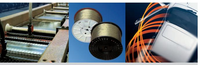
voestalpine Austria Draht GmbH produces wire rod for the manufacture of steel cord car and truck tyres, as well as for bead, tube reinforcement and saw wire. Technologies used in steel production and wire rolling ensure that the wire rod can be drawn down to an extremly thin final size and that the demanding mechanical properties for the finshed product are achieved.
